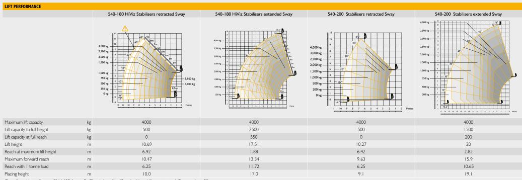
Complies with stability test EN 1459 Annex B. Chassis Levelling (Sway) with stabilisers retracted (Sway angle  $\pm 9^{\circ}$ ).
