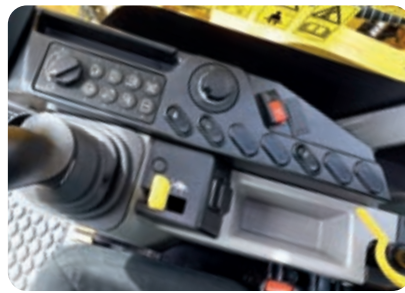
Switches are grouped on the right console for optimal visibility and control
