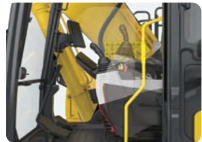
Tiltable side console for safer, more comfortable entry and exit
