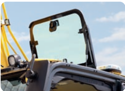
New openable, polycarbonate roof window with sun roller blind
