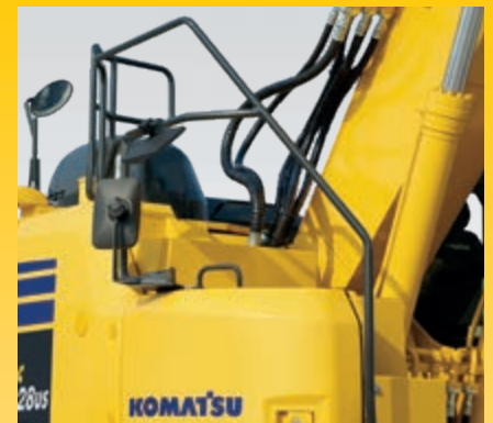
Hand rails and anti-slip plates
