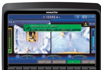
Eco-gauge, Eco guidance and fuel consumption gauge
