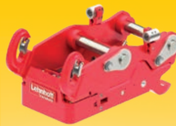
Fully hydraulic quick-coupler Variolock VL100 The operator can comfortably change attachments including hydraulic connections from the cab in a matter of seconds, without having to leave the cab and without depending on other personnel. Leads to increased productivity and encourages the operator to use the right tool for the job. It also helps to prevent hose ruptures and contamination of the hydraulic system and of the environment.
