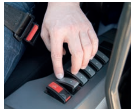
Ergonomically designed switches that light up for safe and easy night operation
