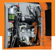
■ Centrally located engine oil filter, pilot and steering filters, and fuel filters allow for quick and easy servicing. Automatic exhaust filter cleaning saves you even more time.
