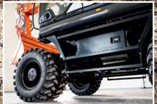
High ground clearance reduces damage from obstacles.
