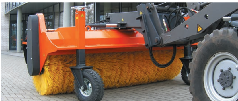
bema Jumbo on a wheel loader (quick change adaptor with roller levelling)
