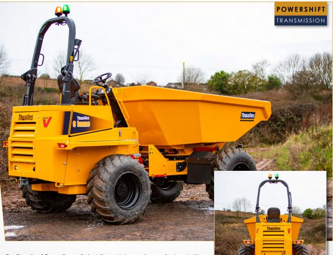
The Thwaites 9 Tonne Power Swivel, Stage V dumper is manufactured with contractors and hirers in mind – ensuring operator safety, reducing risk on site, and improving performance. The Power Swivel skip enables a 90° rotation left and right, allowing the machine easier access to tip loads in restricted areas, giving the operator greater control and reducing risk on site.
