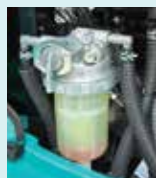
Pre fuel filter with built-in water separator
