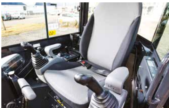
The wide adjustable suspension seat is comfortable for operators.
