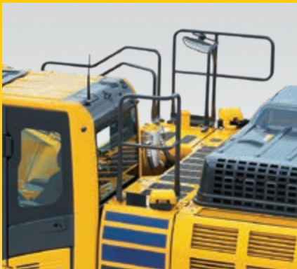
Hand rails and anti-slip plates
