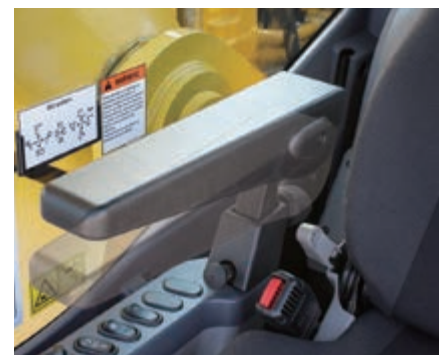
Armrest with simple height adjustment
