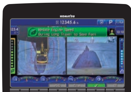
Eco-gauge, Eco guidance and fuel consumption gauge
