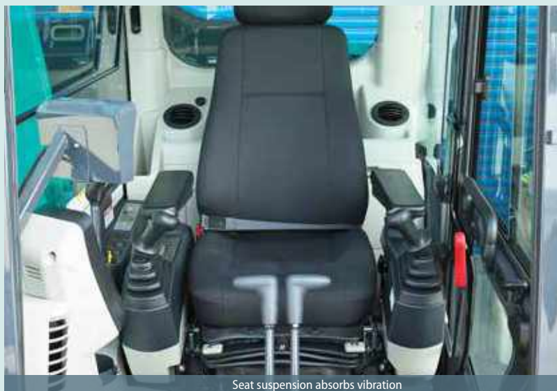
Seat suspension absorbs vibration
