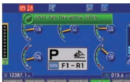
Eco-gauge, Eco guidance and fuel consumption gauge
