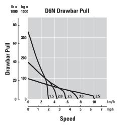
The direct injection electronic fuel system provides a controlled fuel delivery increase as the engine lugs back from rated speed. This results in increased horsepower below rated power. A combination of increased torque rise and maximum horsepower improves response, provides greater drawbar pull and faster dozing cycles.
