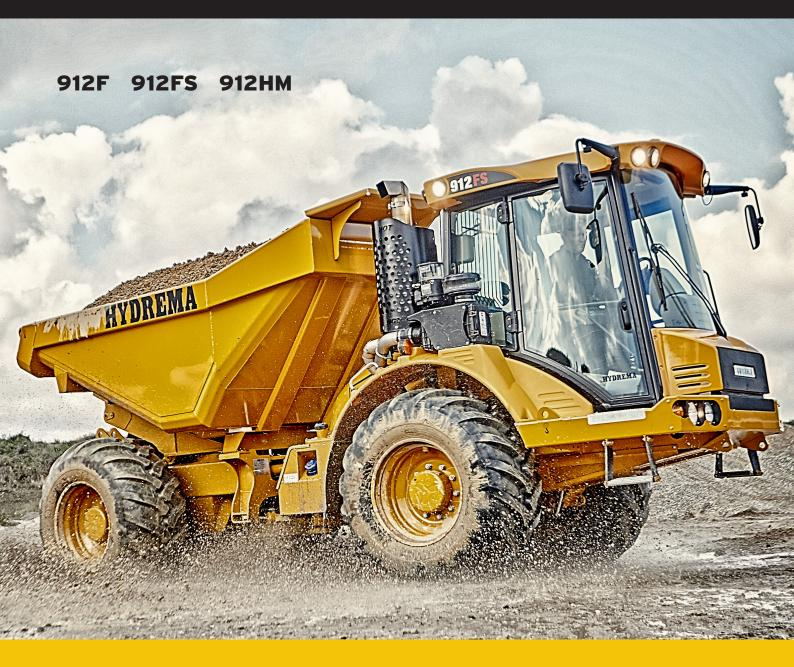
A unique combination of articulated center pivot, wide wheels and high ground clearance - for superior off-road performance.
