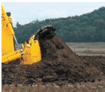
The Sigmaxdozer® blade offers highest material holding capacity
