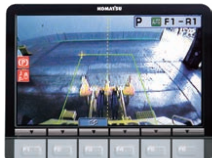
Fully integrated rear-view camera system
