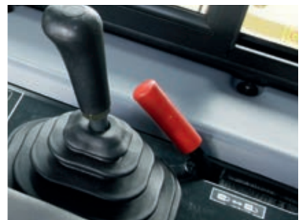
Remote safety lock levers
