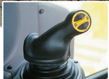
Palm Command Control System (PCCS)
