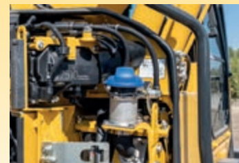
For simple access, the AdBlue® tank is installed on the front stairway.
