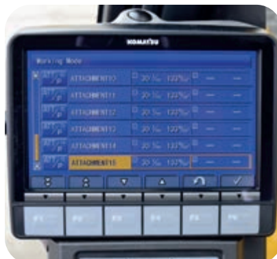
Komatsu Integrated Attachment Control (KIAC) for up to 15 tool presets for oil flow and pressure (option)
