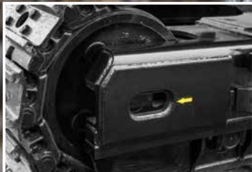
The strengthened motor guard and idler bracket protect against damage.
