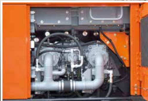
Reduced fuel consumption due to HIOS III B hydraulic technology.
