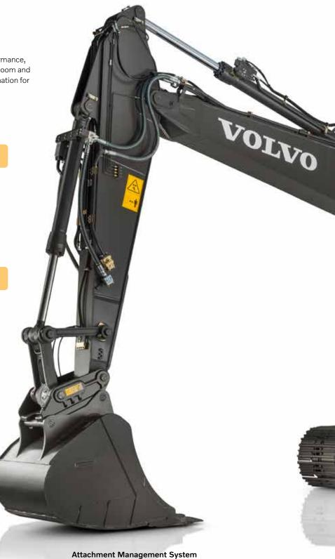
The password protected management system allows storage for up to 20 different attachments. It pre-sets and permits hydraulic flow and pressure to be adjusted within the cab.
