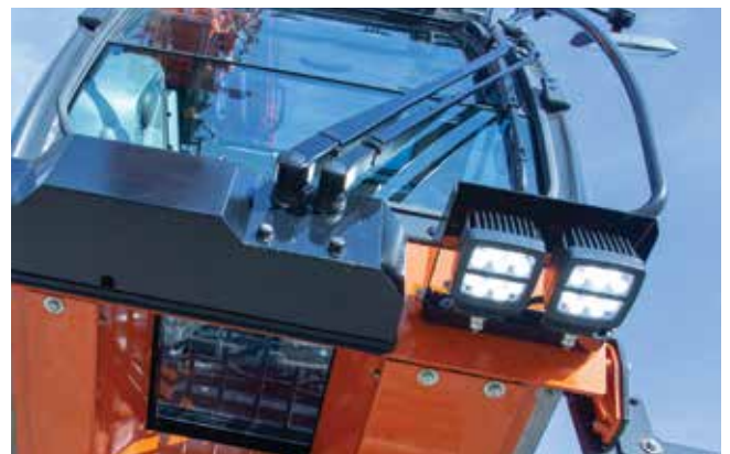
LED lights highlight the working area for operators.
