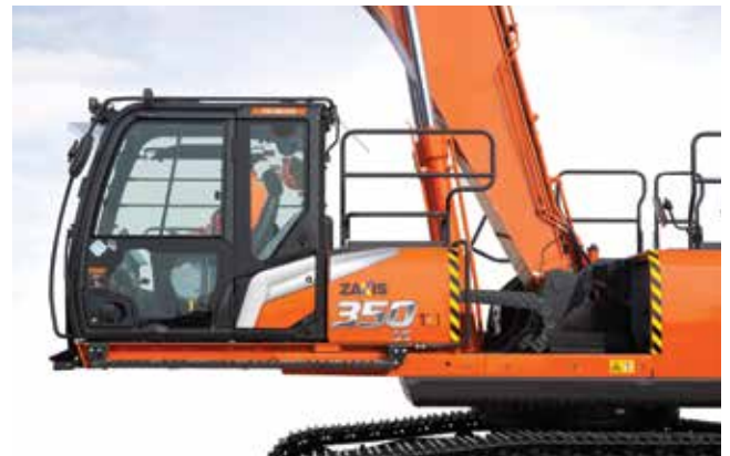
The sliding cab enhances visibility and safety.
