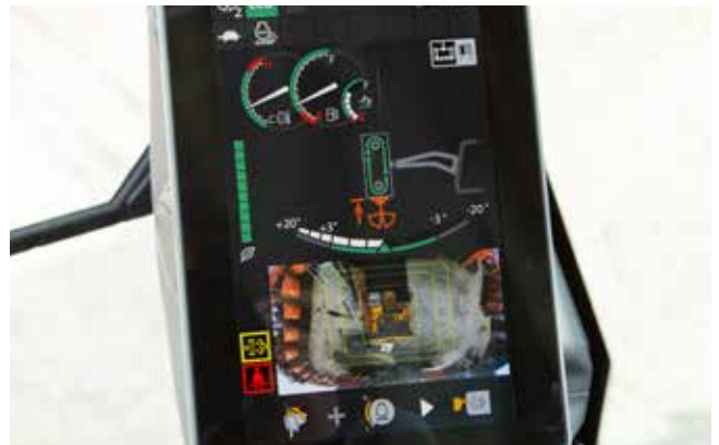
Standard screen includes telescopic indicator display.
